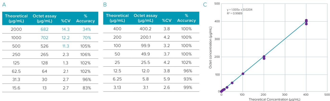
**Figure 1:** Accuracy assessment for the Fab quantitation evaluated in the range 15.6–2000 µg/mL (A) and 3.13–400 µg/mL (B). Linearity of the Fab assay in the range 3.13–400 µg/mL (C). Data in blue on Figure 1A indicate sample concentrations that fall out of specifications for accuracy or % CV.
