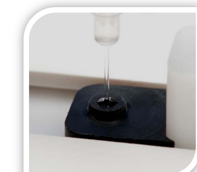
Figure 2: Biosensor testing a 4 µL sample
