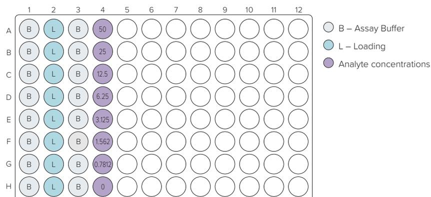
**Figure 2:** An example of a sample plate configuration for an affinity characterization experiment. The “Dip and Read” format allows the user to assay multiple analyte concentrations (purple) in parallel.
