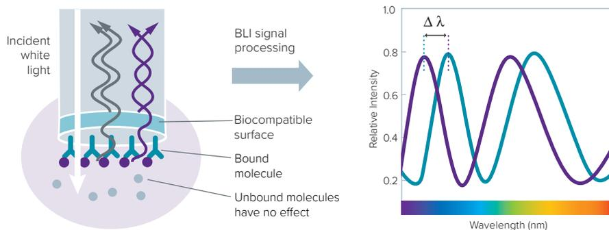
**Figure 1:** Relative intensity of the light reflection pattern from the two surfaces on the biosensor. BLI systems measure the difference in reflected light's wavelength ( $\Delta \lambda$ ) between the two surfaces.
